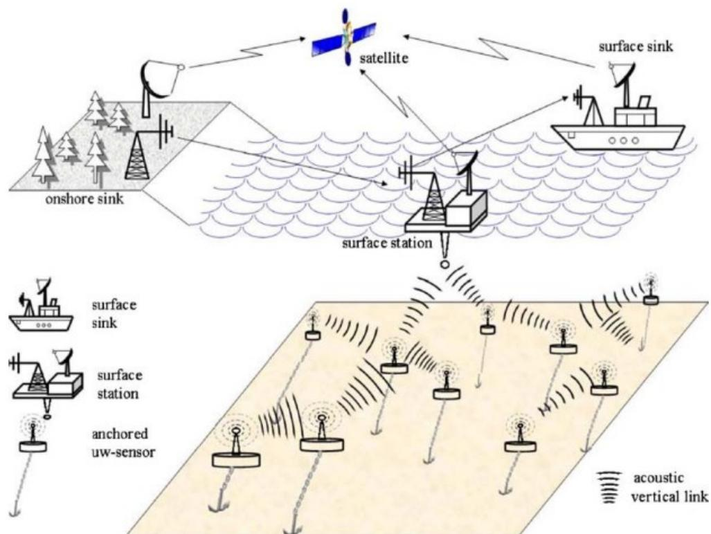
Figure 1. Underwater sensor network architecture (Akyildiz et al., 2005)
