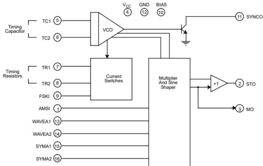
Figure 3. Block diagram of Modulator XR2206
