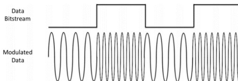
Figure 2. An FSK modulation
