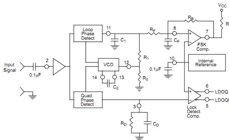
Figure 11. RFSK Demodulator circuit
